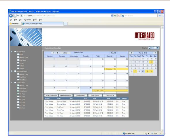
The BACnet schedule manager allows users to define a weekly schedule or exception schedule strategy. The strategy can be saved as a profile for reuse and by selecting the BACnet controllers from the list, write down to each controller with a single operation.
